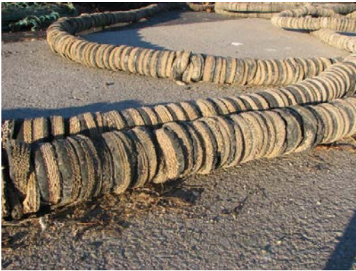
Figure 1 - Ground cable with cookies
